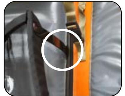
1. Secure left side apron stays into the stay pockets on the Fish Cat 4 Deluxe - LCS. The rear apron stay pocket is located 5" from the front edge of the seat.
