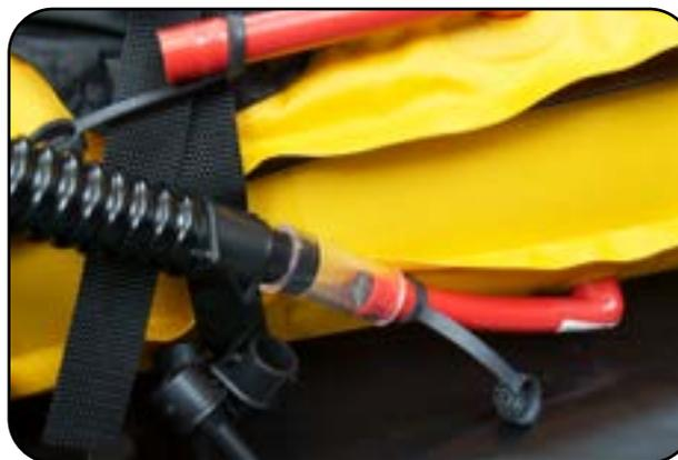
1. Locate the seat bottom inflation tube, connect the hand pump with the vinyl tube adapter and inflate the seat bottom to a firm pressure.
