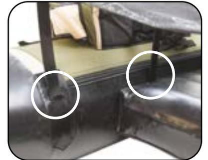
1. Secure left side apron stays into the stay pockets on the Super Fat Cat - LCS. The rear apron stay pocket is located 5" from the front edge of the seat.
